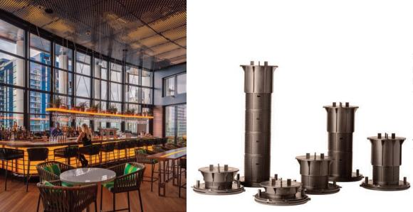
Bison Pedestals are manufactured in Denver, Colorado, USA with 20% postindustrial recycled materials and have patented features that improve performance and stability. Bison Pedestals create level rooftop decks over sloped surfaces and support a variety of different surface materials, including wood, stone, structural porcelain, decorative rock, grating, artificial turf, and concrete to create unique custom looks.
